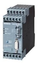
SIPLUS SIMOCODE pro V basic unit 2 based on 3UF7010-1AU00-0 with conformal coating, -25...+60 °C, PROFIBUS DP interface 12 Mbps, RS-485; 4 I/3 O freely parameterizable US: 110-240 V AC/DC; input for thermistor connection; monostable relay outputs; expandable by expansion modules
