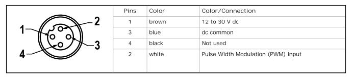
For maximum intensity, leave the white and black wires floating or connected to common.
