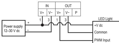
For standard polarity PWM dimming, use with the LC65P2T dimming module. Use the LC65P1T or LC65P1Q5 dimming modules for opposite polarity dimming.
