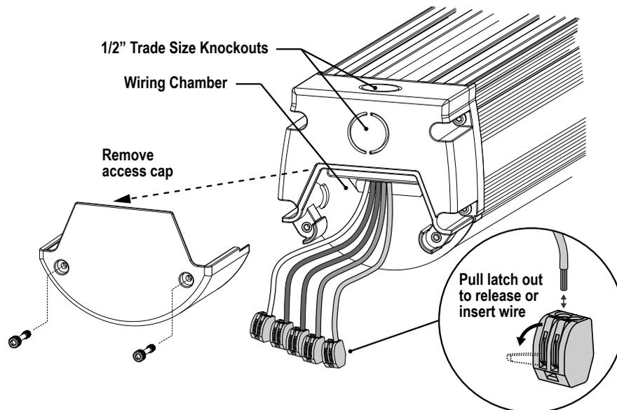
1. Loosen the screws to remove the access cap from the wiring chamber.
