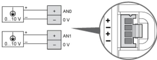
The (-) poles are connected internally.
