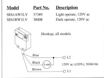
mounted indicator LED that lights whenever the sensor is seeing the modulated light beam. Sensors use 3-wire ac hookup. See hookup, above right.
