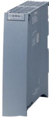
SIMATIC S7-1500, digital input module, DI 64xDC 24V SNK/SRC BA, 64 channels in groups of 16, input delay typ. 3.2 ms, input type 3 (IEC 61131); sinking/sourcing input. 35 mm wide, cables and terminal blocks to be ordered separately as accessories
