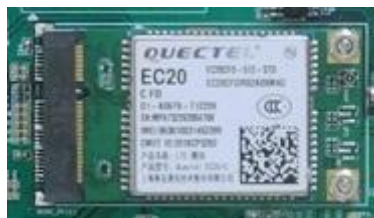
Figure 596: mini-PCle Connector & 4G Module
