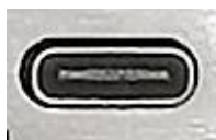
USB Type-C Port (embedded / enclosed PC version)
