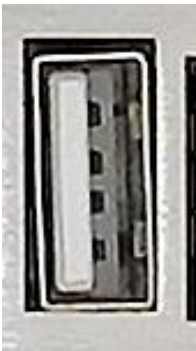
USB 2.0 HOST Port (embedded / enclosed PC version)
