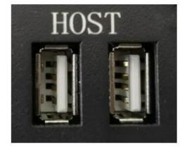
Figure 966: USB HOST Connectors (embedded/enclosed PC version)
