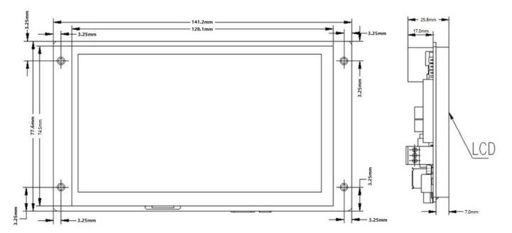
Figure 975: CS12720RA4050E Technical Drawing
