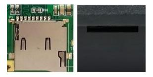
Figure 970: TF (micro SD) Card Slot
