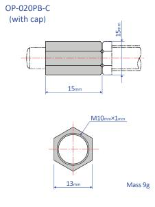
Note: When attaching, make sure that the side without a bearing chamfer is the impact surface.
