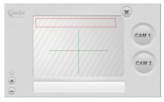
The HMI screen is composed out of 6 touchable buttons, 2 text zones, a red rectangle, and two lines (green and blue). All of these elements have been placed with the HMI Editor of GraphConverter.
