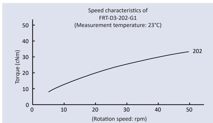
■ **Speed characteristics:** A rotary damper's torque varies according to the rotation speed. In general, as shown in the graph above, the torque increases as the rotation speed increases, and the torque decreases as the rotation speed decreases. In addition, please note that the starting torque slightly differs from the rated torque.
