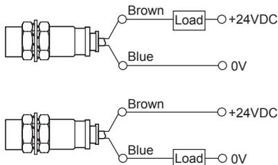
※Load can be wired to any direction.
