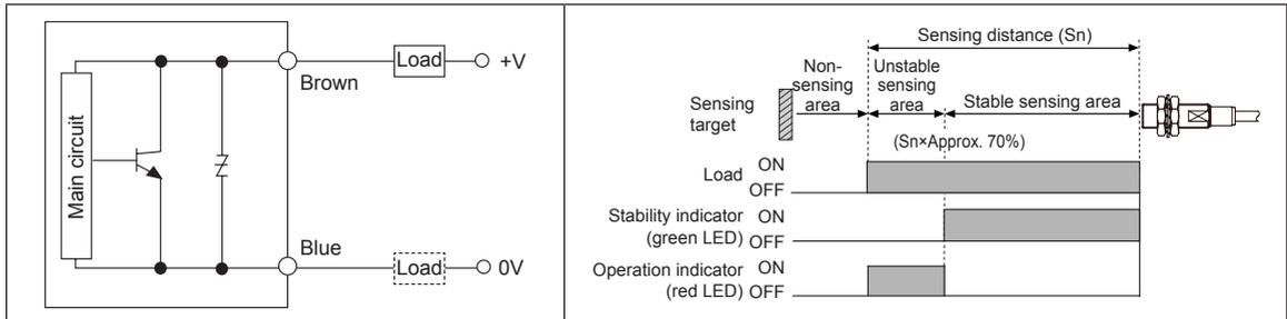
※When the sensing target is placed over approx. 70% of sensing distance ( $S_n$ ), the operation indicator (red LED) turns ON. When the target is placed within approx. 70% of sensing distance ( $S_n$ ), the stability indicator (green LED) turns ON. Use the sensor at the position where the stability indicator turns ON.
