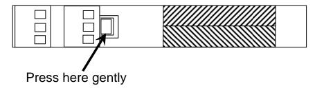
There are 4 switch banks, S1, S2, S3 and S4, located inside the SC-DUALCON as shown below:
