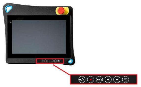
The TP-100-C's membrane keys are located at the lower-right of the teach pendant, each membrane key is mapping to the real-keyboard signal, review the key definitions below:
