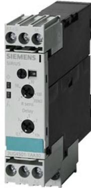
Analog monitoring relay Fill level monitoring Resistance monitoring from 2 to 200 kohm Overshoot and undershoot Supply voltage 24 V AC/DC 50 to 60 Hz DC and AC without galvanic isolation to measuring circuit 2-step or 1-step control Tripping delay 0.5 to 10 s 1 change-over contact screw terminal Successor product for 3UG3501-1AC20
