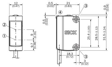
① Center of optical axis, sender
