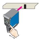
When setting the contrasts to be detected, the second LED (green) flashes in the bar graph. Press set button. The Quality of Teach is displayed.
