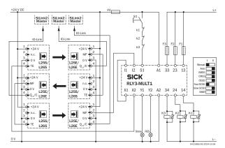
The specifications in the operating instructions for the devices used must be followed.  $3 \times L25/L26$  to RLY3-MULT1, with restart interlock and external device monitoring
