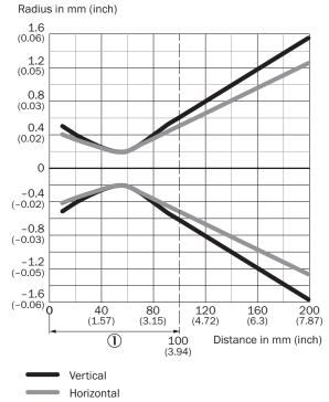
① Minimum distance between sensor and reflector
