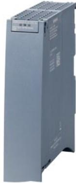
SIMATIC S7-1500, digital output module, DQ 64xDC 24V/0.3A SNK BA, 64 channels in groups of 16, 2 A per group at 60 °C, sourcing output, 35 mm wide cables and terminal blocks to be ordered separately as accessories
