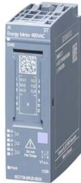
\*\*\* spare part \*\*\* SIMATIC ET 200SP, Analog input module, AI Energy Meter 480 V AC ST, suitable for BU type D0, channel diagnostics
