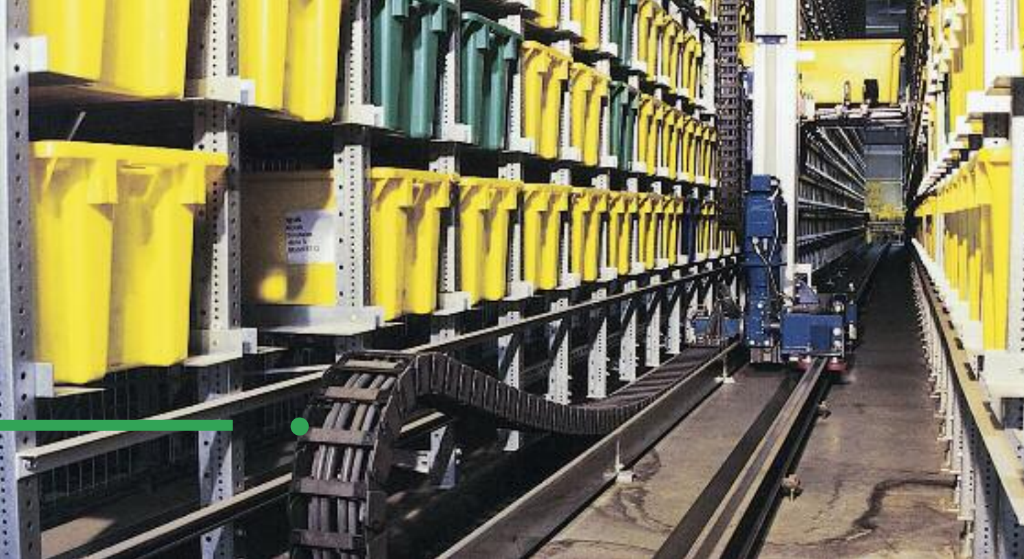
Series 350 Energy Chain®, steel guide trough and Chainflex cables used in a shelf conveyor application
