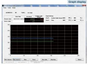
Change in current values can be plotted on a chart and the amount of change can be checked over time.
