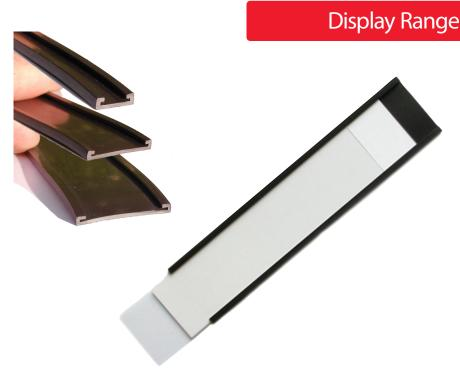
The Labelling Holder has three parts. The C-shaped magnetic extrusion is multiple poled magnetic at the rear. A White Card fits within the profile slot and this can be written upon or labels could be added to it as necessary to display the Sign or Information. Then a Clear Plastic Cover (PVC) fits over the White Card within the profile to protect the White Card from dirt to complete the Magnetic Labelling Holder.
