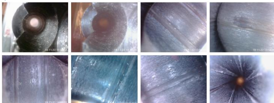
Interior of gun barrel as seen from a GB-430/460:
