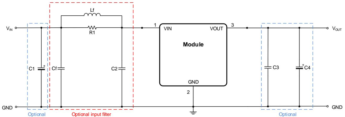
The 173950x78 integrates both the input and output capacitors. Therefore, additional external input/output capacitors are normally not required.
