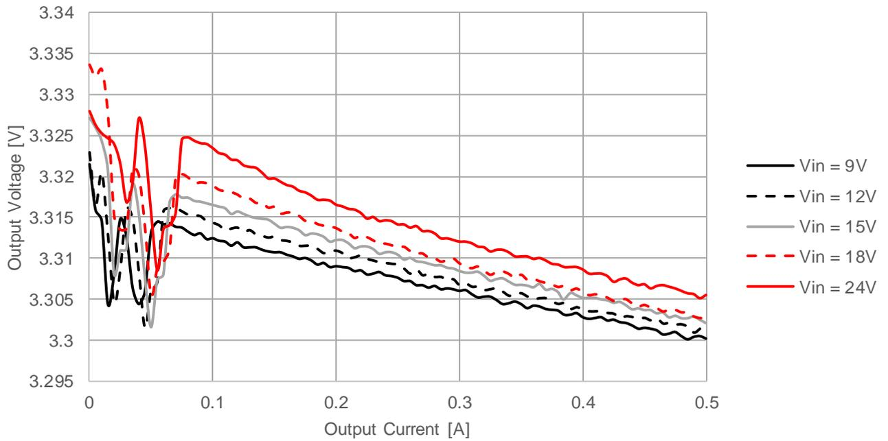
173950378 Load Regulation  $V_{OUT}=3.3V$ ,  $T_A = 85^\circ C$
