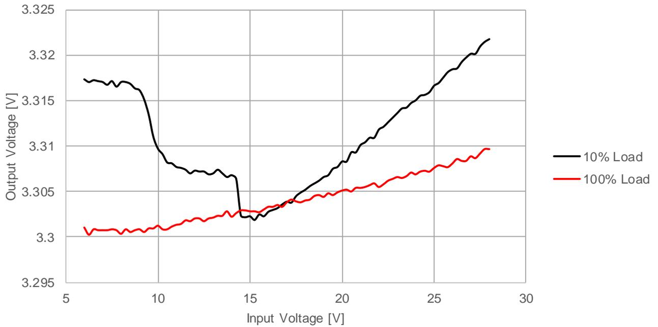
173950578 Line Regulation  $V_{OUT} = 5V$ ,  $T_A = 25^\circ C$
