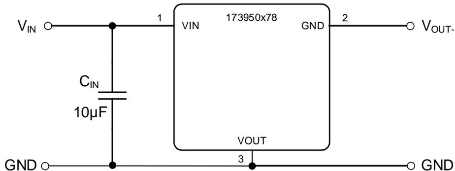
It is important to be aware that in this configuration the 173950x78 must withstand the sum of the input voltage and the absolute value of the output voltage ( $V_{IN} + |V_{OUT}|$ ), instead of just the input voltage. This means that the maximum operating voltage should be limited to  $28V - |V_{OUT}|$  (e.g. if the 173950x78 is used in this configuration, the input voltage should not exceed 23V).
