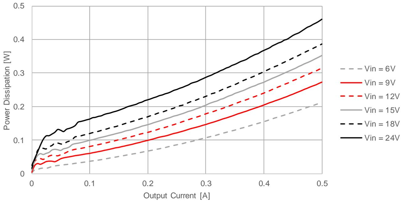
173950378  $V_{OUT} = 3.3V$ ,  $f_{SW} = 570kHz$ ,  $T_A = 85^\circ C$
