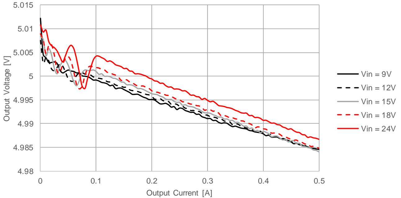
173950578 Load Regulation  $V_{OUT}=5V$ ,  $T_A = 85^\circ C$
