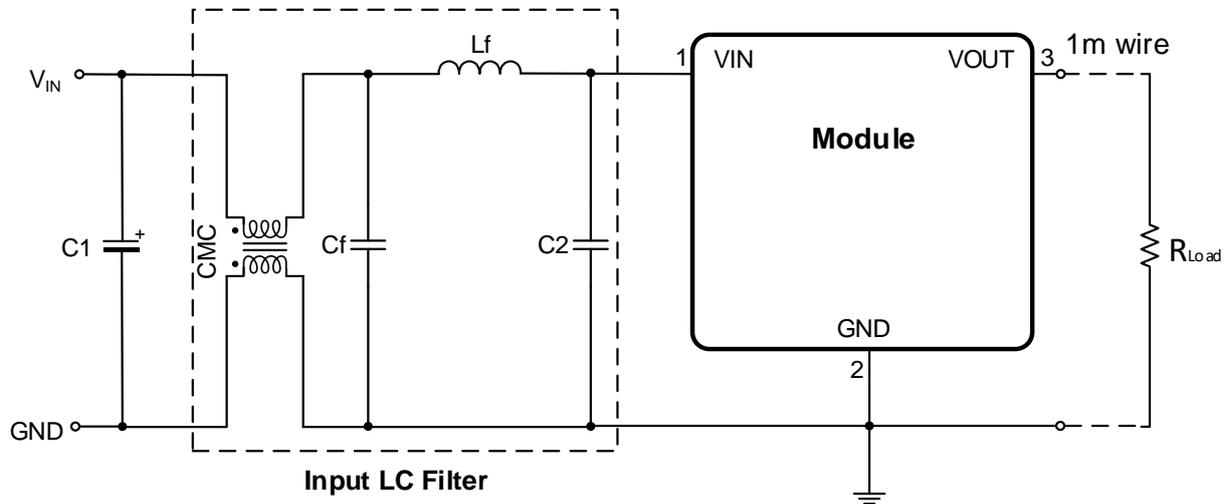
**Bill of Material of the Input LC Filter (V<sub>IN</sub> = 24V, V<sub>OUT</sub> = 3.3V and 5V, I<sub>OUT</sub> = 500mA)**
