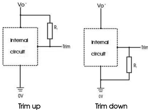
TRIM resistor connection (dashed line shows internal resistor network)
