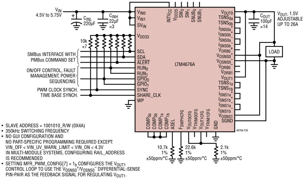
Figure 35. 26A, 1.5V Output DC/DC μModule Regulator with I<sup>2</sup>C/SMBus/PMBus Serial Interface
