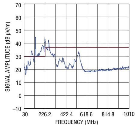
**Figure 32. Radiated Emissions Scan of the LTM4676A Producing 1V<sub>OUT</sub> at 26A, from 12V<sub>IN</sub>. DC1811B-B Hardware with Outputs Paralleled. No Snubbers Applied.  $f_{SW} = 350$ kHz. Measured in a 10m Chamber. Peak Detect Method**
