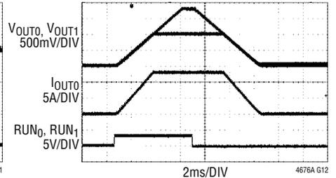
FIGURE 69 CIRCUIT AT  $12\text{V}_{\text{IN}}$ .  $77\text{m}\Omega$  LOAD ON  $\text{V}_{\text{OUT}0}$ . NO LOAD ON  $\text{V}_{\text{OUT}1}$ .  $\text{TON\_RISE}_0 = 3\text{ms}$ ,  $\text{TON\_RISE}_1 = 5.297\text{ms}$ ,  $\text{TOFF\_DELAY}_1 = 0\text{ms}$ ,  $\text{TOFF\_DELAY}_0 = 2.43\text{ms}$ ,  $\text{TOFF\_FALL}_1 = 5.328\text{ms}$ ,  $\text{TOFF\_FALL}_0 = 3\text{ms}$ ,  $\text{ON\_OFF\_CONFIG}_0 = 0\text{x}1\text{E}$
