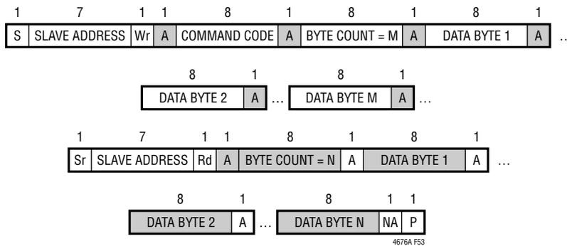
Figure 59. Block Write – Block Read Process Call
