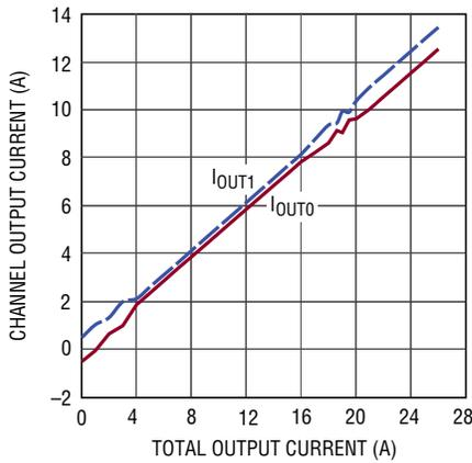
(36a) 5V<sub>IN</sub>, Figure 35 Circuit
