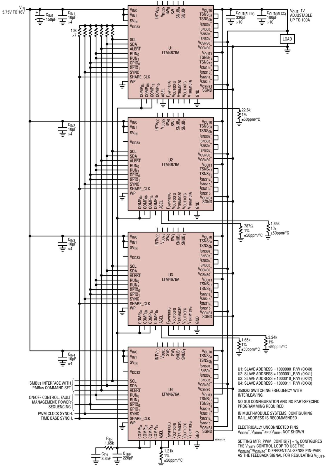
Figure 39. Four Paralleled LTM4676A Producing 1V<sub>OUT</sub> at up to 100A. Integrated Power System Management Features Accessible Over 2-Wire I<sup>2</sup>C/SMBus/PMBus Serial Interface. Evaluated on DC1989B-C
