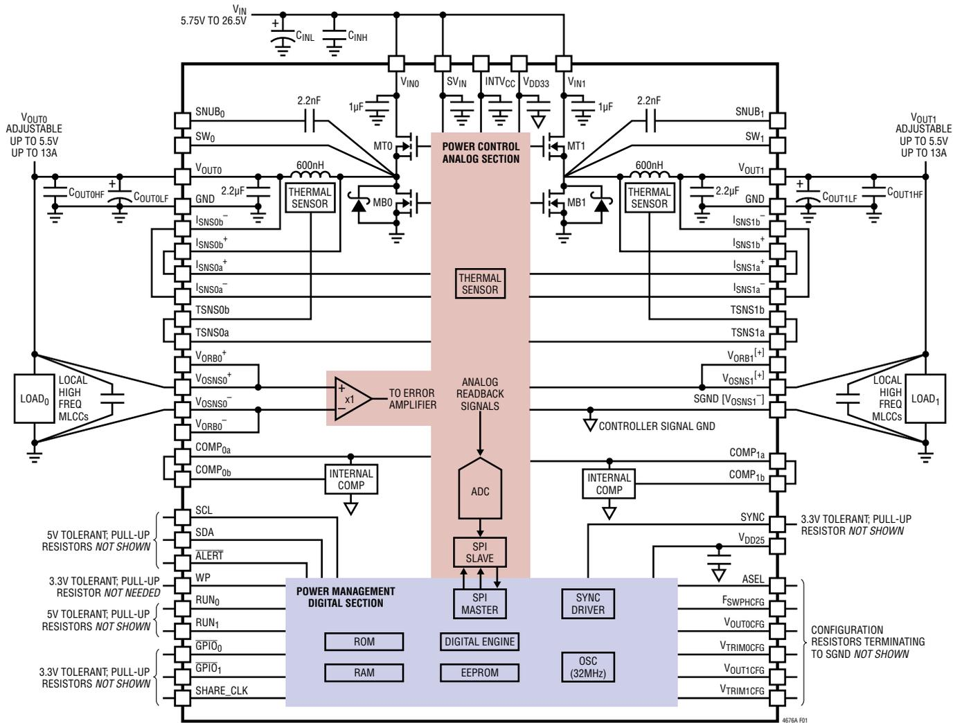
Figure 1. Simplified LTM4676A Block Diagram
