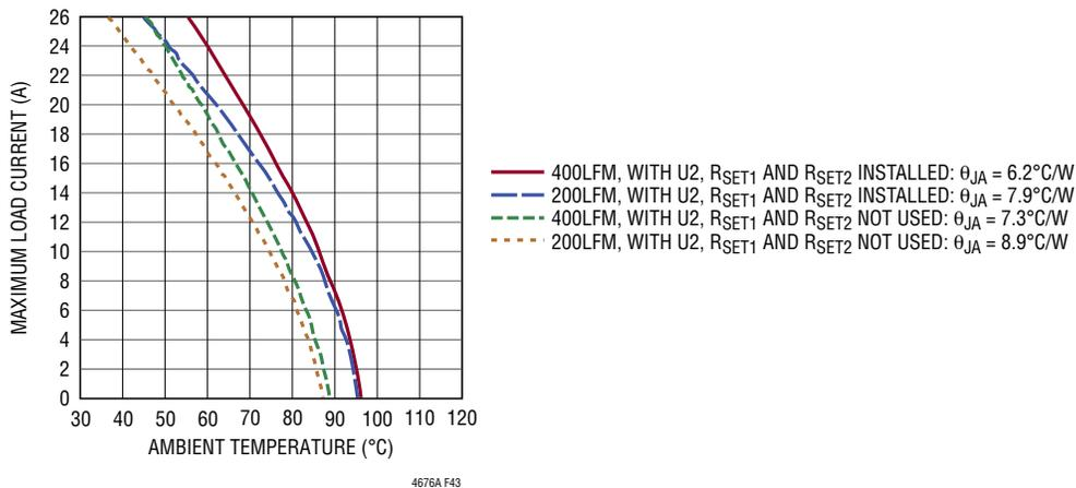
Figure 43. Output Derating Curve of Figure 42 Circuit Tested on DC1811B-B, 12V<sub>IN</sub>, No Heat Sink
