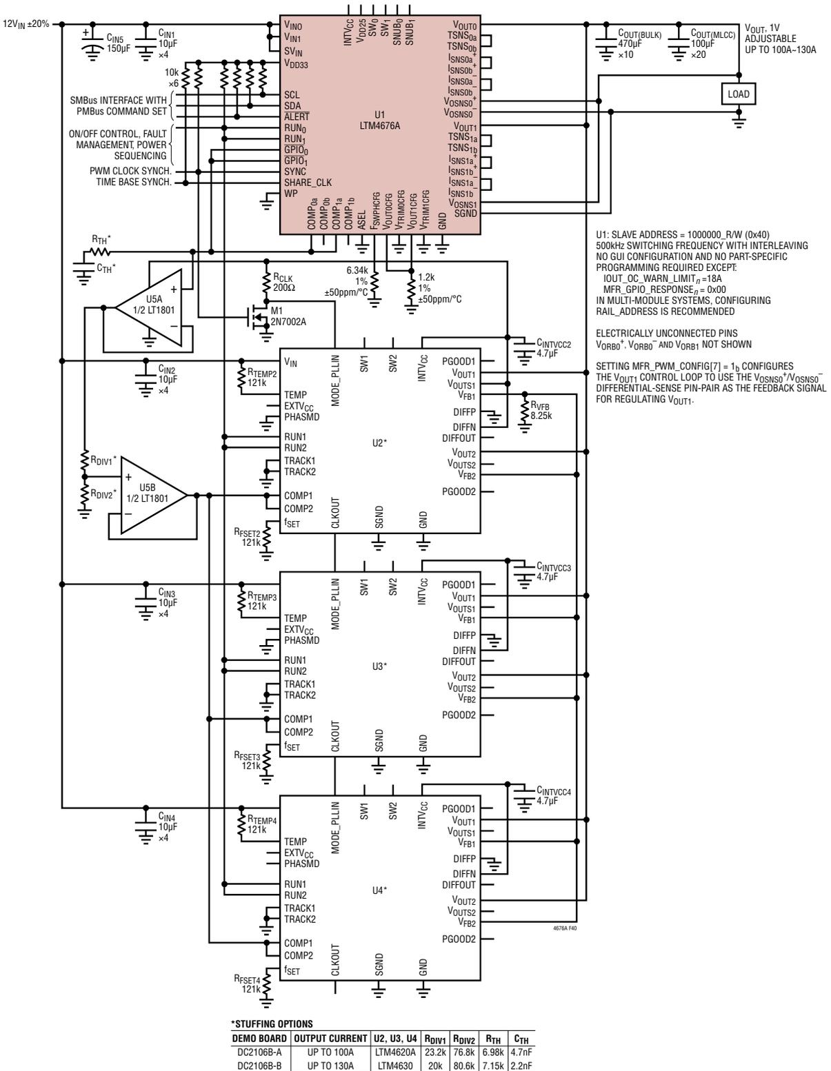
Figure 40. One LTM4676A Operating In Parallel with 3xLTM4620A or 3xLTM4630 (See Demo Boards DC2106B-A, DC2106B-B) Producing 1V<sub>OUT</sub> at up to 100A ~ 130A. Power System Management Features Accessible Through LTM4676A. See Figure 41
