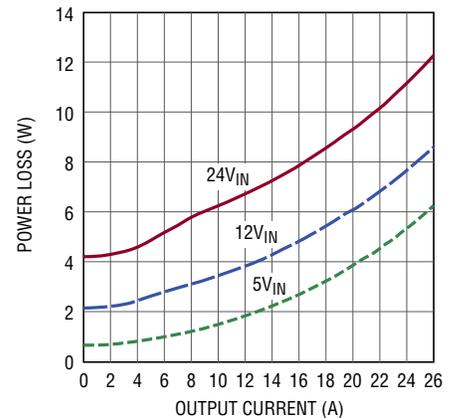
Figure 13. 3.3V<sub>OUT</sub> Power Loss Curve
