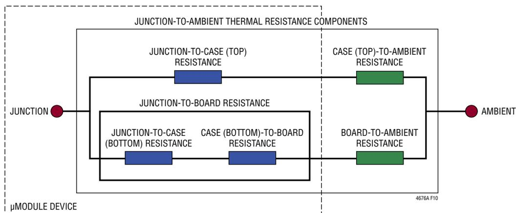
Figure 10. Graphical Representation of JESD51-12 Thermal Coefficients
