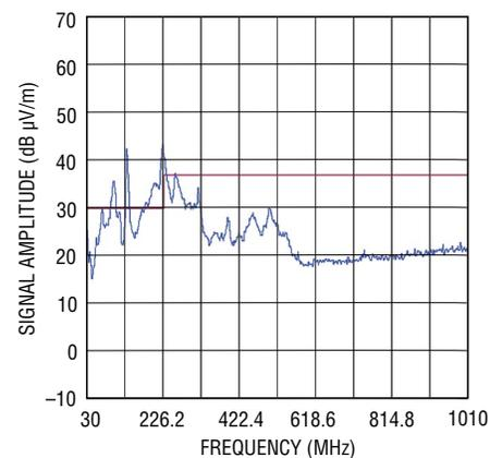
**Figure 33. Radiated Emissions Scan of the LTM4676A Producing 1V<sub>OUT</sub> at 26A, from 12V<sub>IN</sub>. DC1811B-B Hardware with Outputs Paralleled. 1 $\Omega$  (1/4W rated) Snubber Resistors Applied from  $SNUB_n$  to GND.  $f_{SW} = 350$ kHz. Measured in a 10m Chamber. Peak Detect Method**
