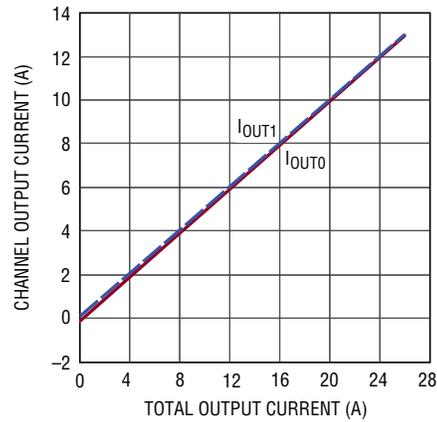
(36b) 12V<sub>IN</sub>, Figure 35 Circuit with INTV<sub>CC</sub> Open and V<sub>OUT</sub> Commanded to 1V
