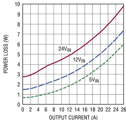
Figure 12. 1.8V<sub>OUT</sub> Power Loss Curve
