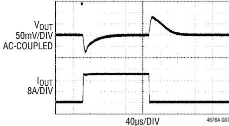
FIGURE 35 CIRCUIT AT  $12\text{V}_{\text{IN}}$ .  $\text{INTV}_{\text{CC}}$  PIN OPEN CIRCUIT AND  $\text{VOUT\_COMMAND}_0$  SET TO  $1.000\text{V}$ .  $0\text{A}$  TO  $20\text{A}$  LOAD STEP AT  $20\text{A}/\mu\text{s}$
