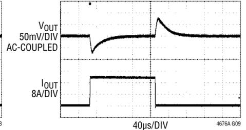
FIGURE 35 CIRCUIT AT  $5\text{V}_{\text{IN}}$ .  $\text{VOUT\_COMMAND}_0$  SET TO  $1.000\text{V}$ .  $0\text{A}$  TO  $20\text{A}$  LOAD STEP AT  $20\text{A}/\mu\text{s}$
