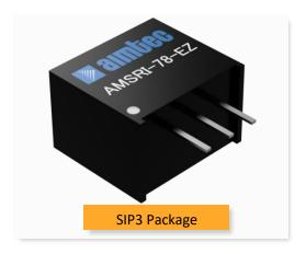
The AMSRI-78-EZ series are SIP3 DC/DC high efficiency switching regulators and ideal substitutes for LM78xx series three-terminal linear regulators. The switching regulators feature high efficiency, low loss, short circuit protection, and there is no need for a heat sink.
