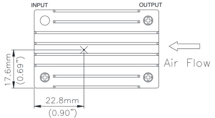
**Figure 16:** Hot spot 1 temperature measurement location
