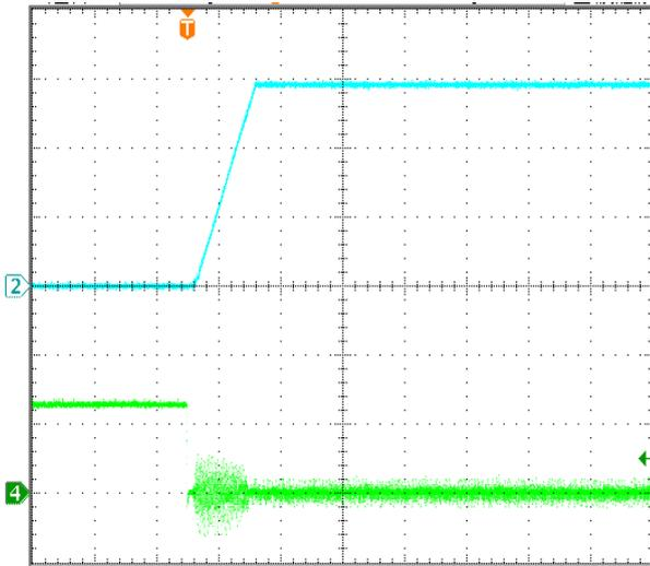
**Figure 4: Remote On/Off (negative logic) at full load**
