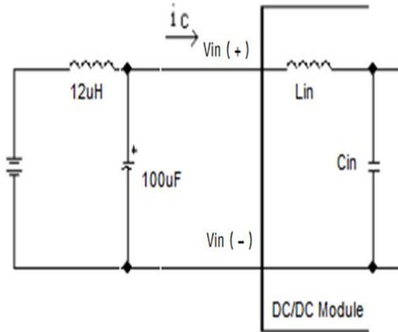
**Figure 8: Test Setup Diagram for Input Ripple Current**
