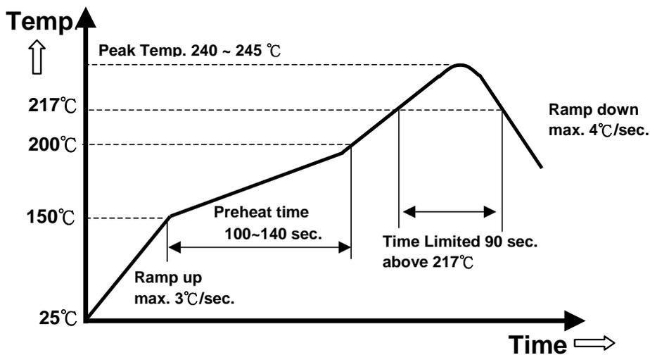
Recommended Temperature Profile for Lead-free Reflow Soldering
