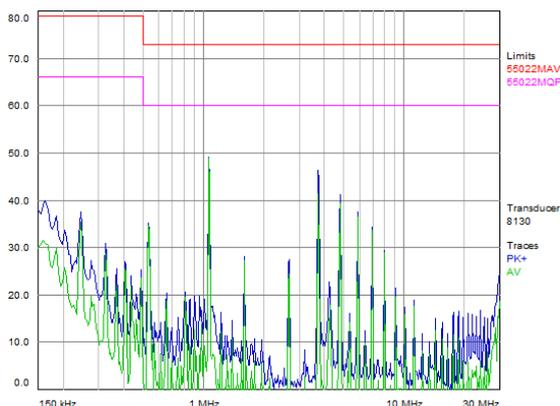
Figure 12-2: Test Result of EMC ( $V_{in}=54V$ ,  $I_o=51A$ ).
