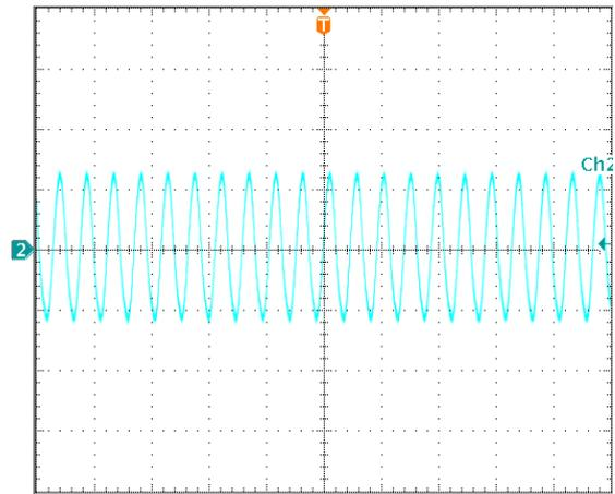
**Figure 11: Output Voltage Ripple and Noise** at nominal input voltage and max load current (20 mV/div, 2us/div)
