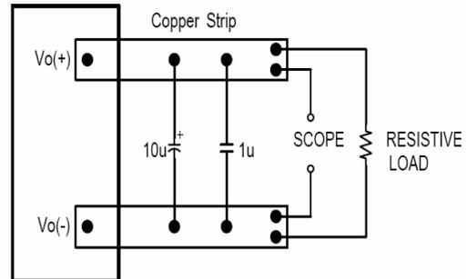
Output voltage ripple test setup.
