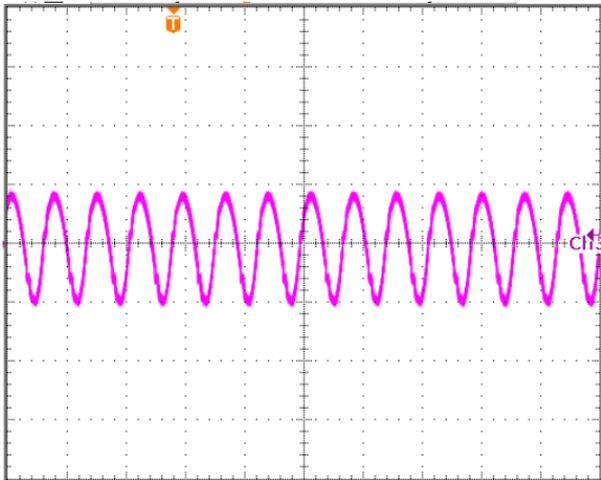
Input Terminal Ripple Current,  $i_c$ , at full rated output current and nominal input voltage with  $12\mu\text{H}$  source impedance and  $100\mu\text{F}$  electrolytic capacitor (250 mA/div, 4us/div).
