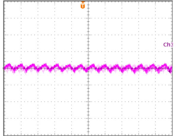
Input reflected ripple current,  $i_s$ , through a  $12\mu\text{H}$  source inductor at nominal input voltage and rated load current (25 mA/div, 4us/div)
