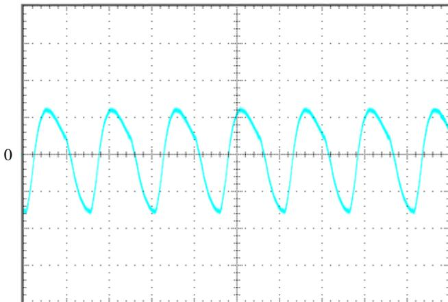
Output voltage ripple at nominal input voltage and max load current
