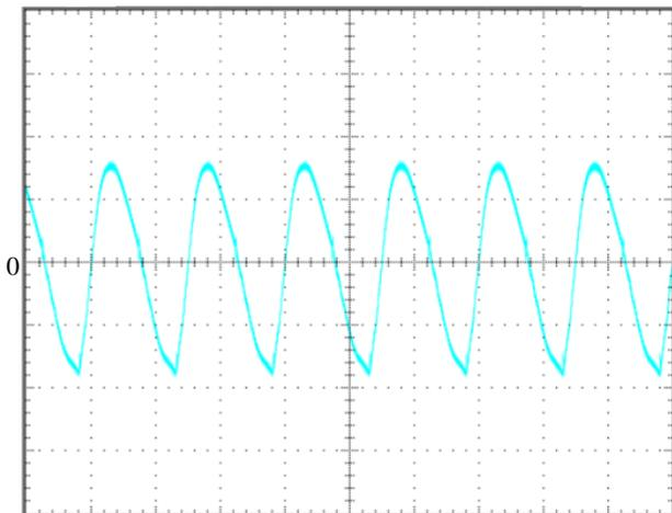
Output voltage ripple at nominal input voltage and max load current
