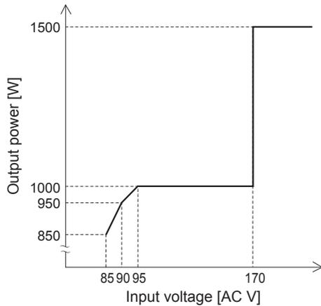
Output voltage derating curve
