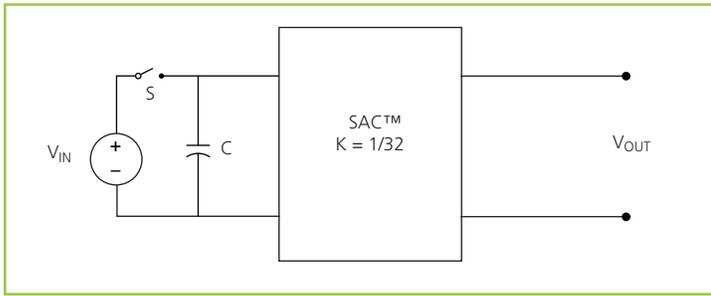
**Figure 19** — Sine Amplitude Converter™ with input capacitor
