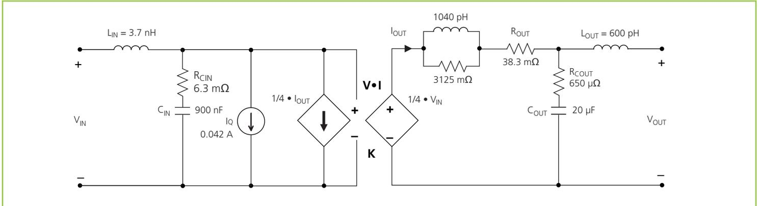
Figure 17 — VI Chip® module AC model
