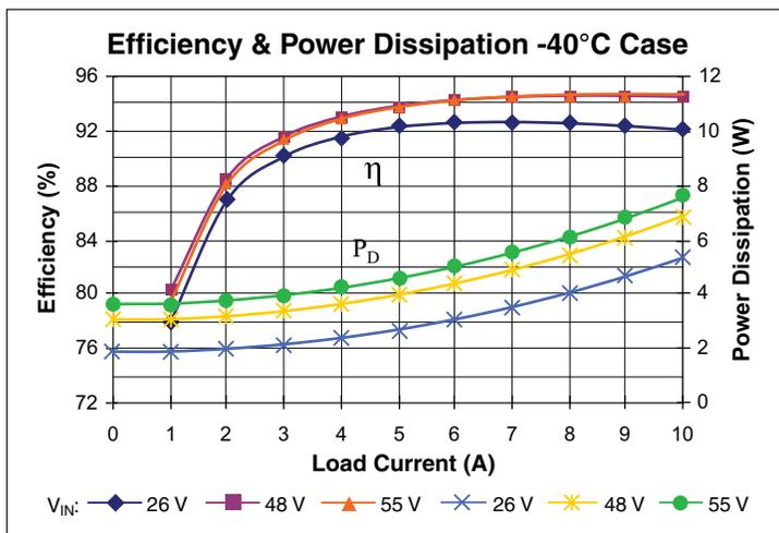
Figure 3 — Efficiency and power dissipation at  $-40^\circ\text{C}$
