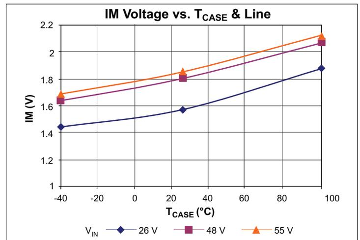
Figure 10 — Full load IM voltage vs.  $T_{CASE}$
