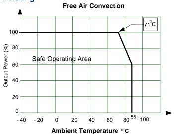
NOTE: With air convection speed of 0.8m/sec
