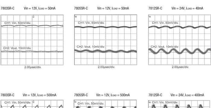
Noise and Ripple - 10% and 100% Load, 20MHz Bandwidth
