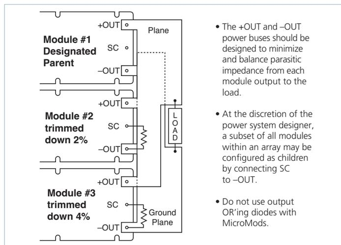
Figure 11 — N+1 module array output connections
