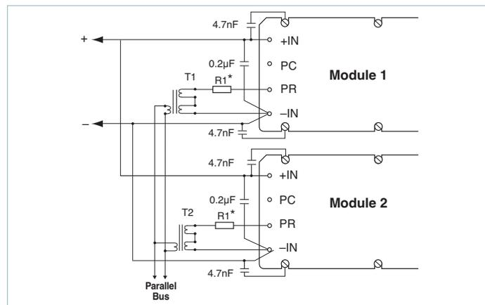
Figure 10 — Transformer-coupled interface
