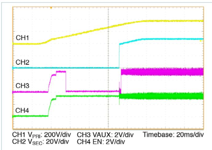
**Figure 17** — Start up from application of  $V_{PRI\_DC} = 380V$ , 50%  $I_{SEC\_DG}$
