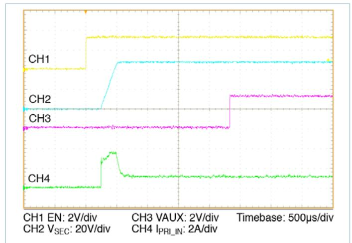
**Figure 18** — Start up from application of  $EN$  with pre-applied
