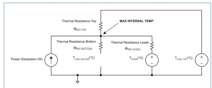
Figure 23 — Top case and leads thermal model
