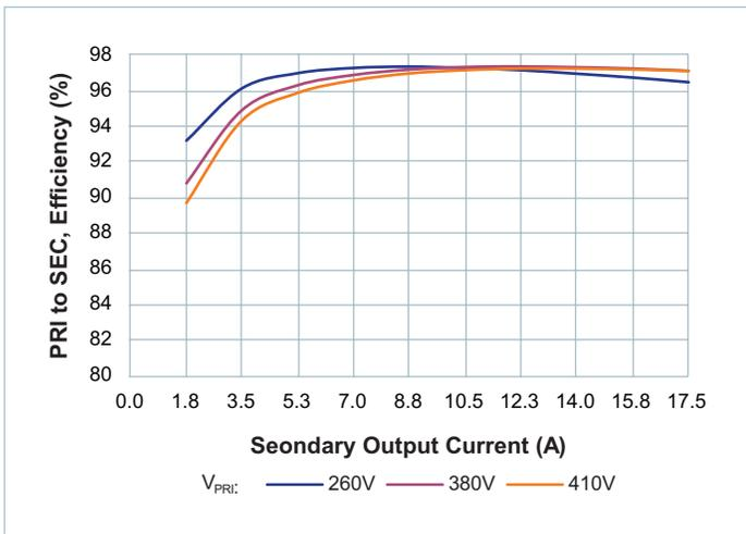
Figure 10 — Efficiency at  $T_{CASE} = 90^{\circ}C$
