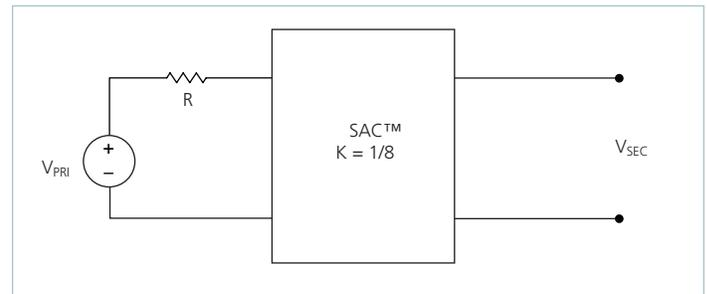
Figure 20 — K = 1/8 Sine Amplitude Converter with series primary resistor
