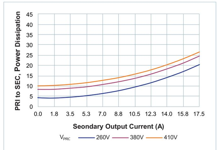
Figure 11 — Power dissipation at  $T_{CASE} = 90^{\circ}C$
