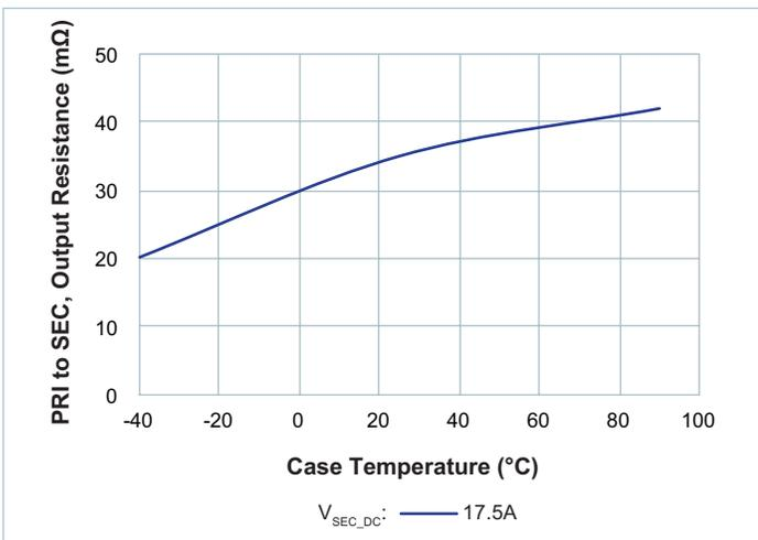
Figure 12 —  $R_{SEC}$  vs. temperature; Nominal  $V_{PRI\_DC}$
