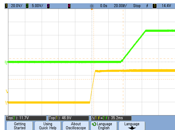
Figure 21. Vin Start-up Delay (CH2: Vout, CH1: Vin) (Vin=48V, Iload=33A, Cload=5500μF, Ta=+25°C, 20mS/div)
