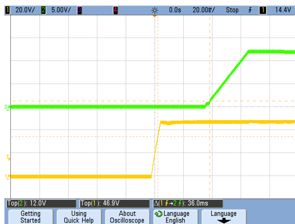
Figure 20. Vin Start-up Delay (CH2: Vout, CH1: Vin) (Vin=48V, Iload=0A, Cload=5500μF, Ta=+25°C, 20mS/div)
