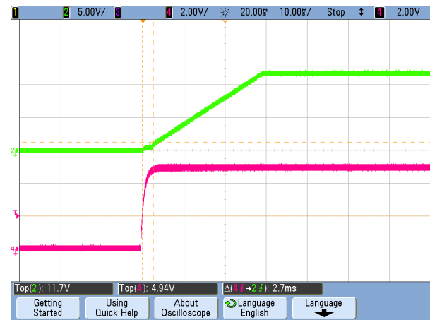
Figure 21. Vin Start-up Delay (CH2: Vout, CH1: Vin) (Vin=48V, Iload=33A, Cload=5500μF, Ta=+25°C, 20mS/div)
