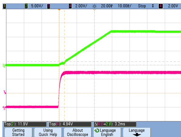
Figure 20. Vin Start-up Delay (CH2: Vout, CH1: Vin) (Vin=48V, Iload=0A, Cload=5500μF, Ta=+25°C, 20mS/div)
