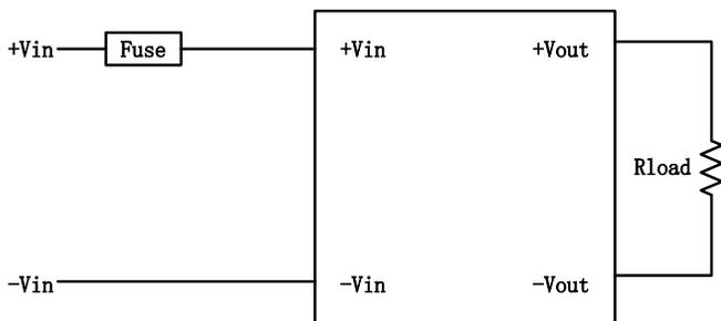
**Figure 2. Input Fusing**
