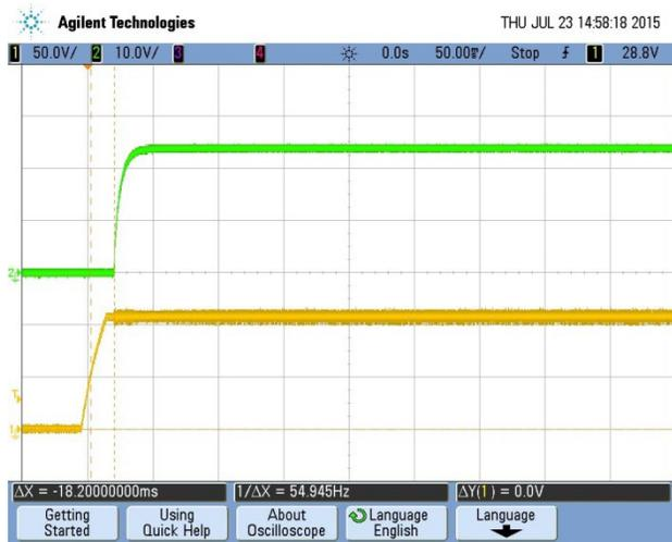
**Turn-on transient at zero load current**
