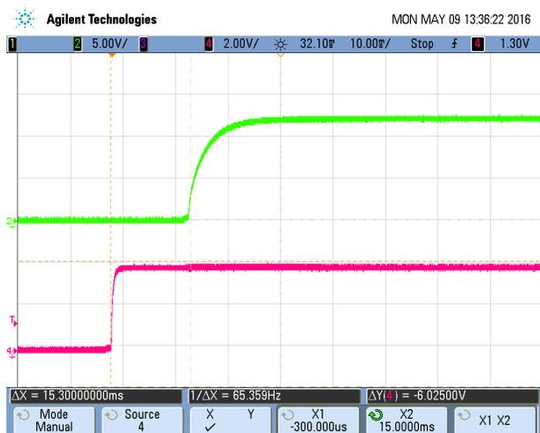
Turn-on transient at zero load current
