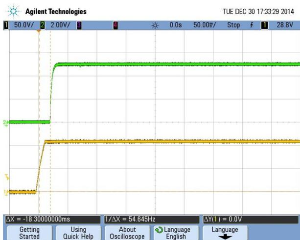
Turn-on transient at zero load current
