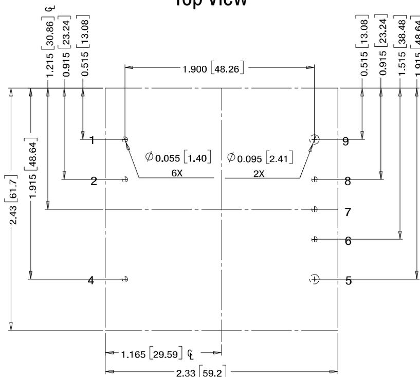
Recommended Footprint for Slotted / Flanged Baseplate and Standard Baseplate
