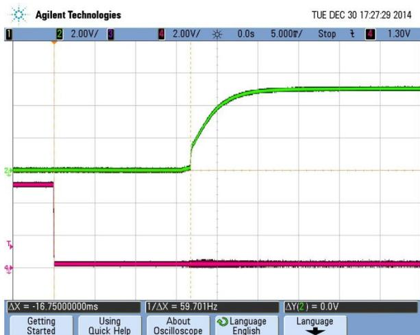
Turn-on transient at zero load current
