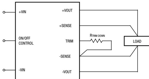
**Figure 8 Trim Connections to Decrease Output Voltage**
