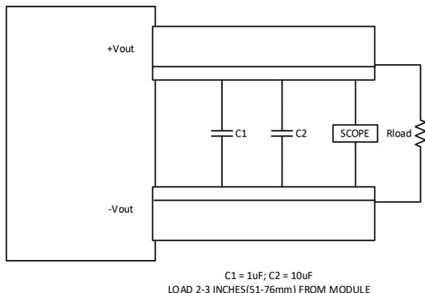
**Figure 4 Measuring Output Ripple and Noise (PARD)**
