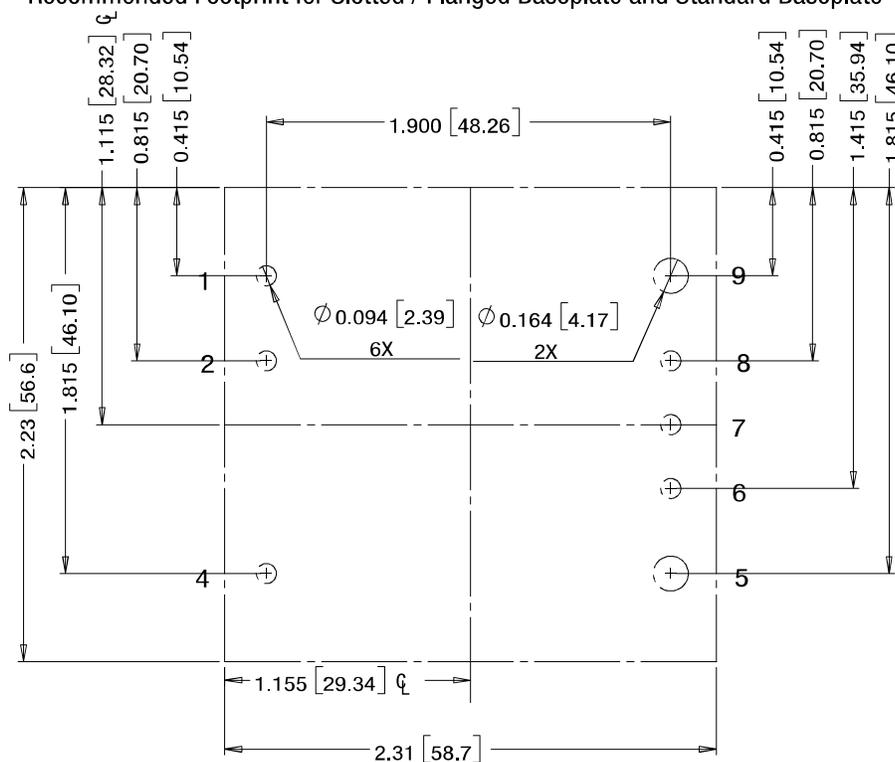
Recommended Footprint for "V" Option Pins / Pinout with Slotted / Flanged Baseplate
