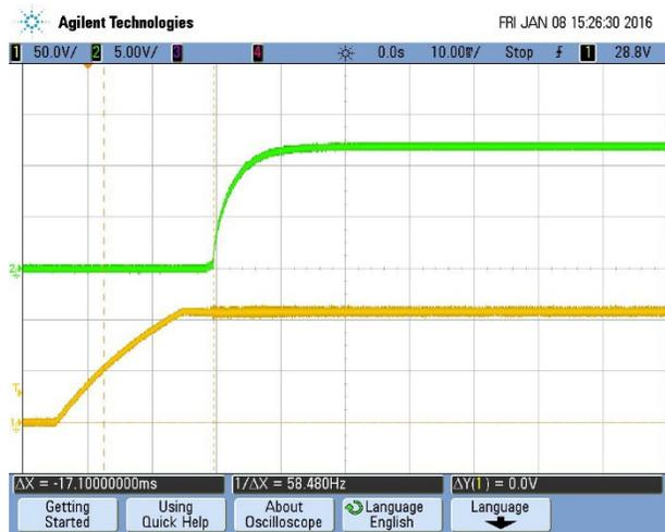
Turn-on transient at zero load current
