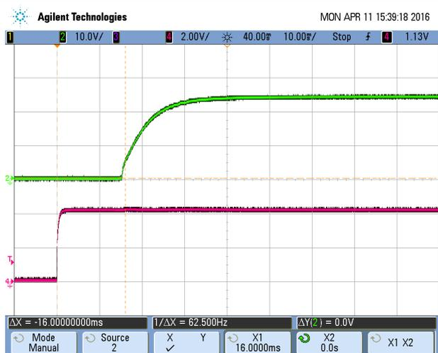
**Turn-on transient at zero load current**
