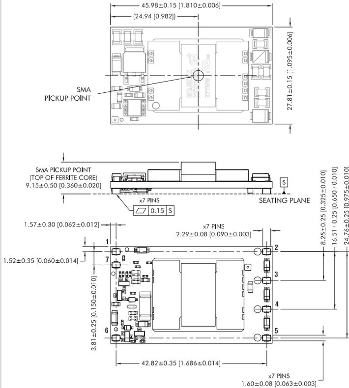
All dimensions in mm (inches), Controlling dimensions is mm.
