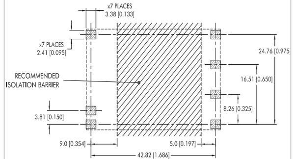
All dimensions in mm (inches), Controlling dimensions is mm.
