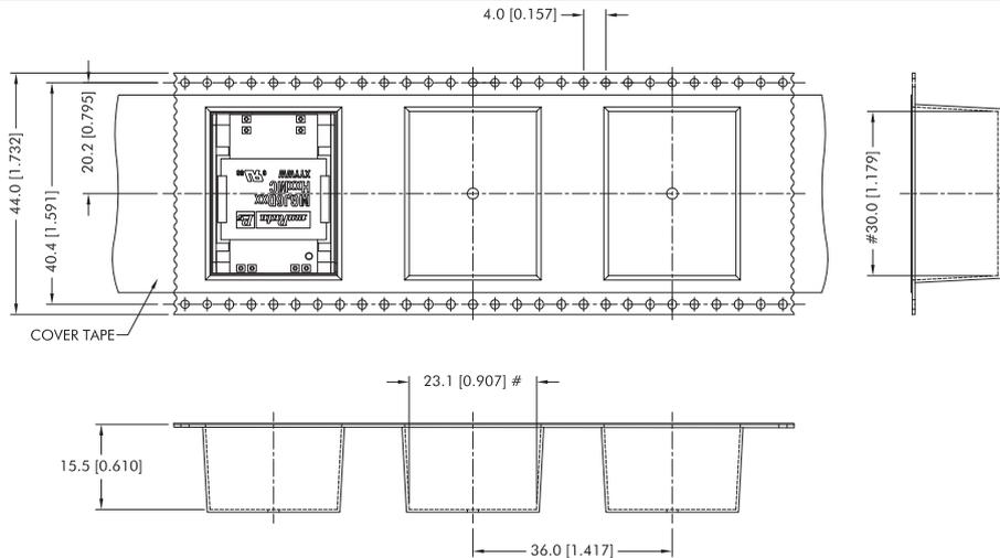
Tape & Reel specifications shall conform with current EIA-481 standard
