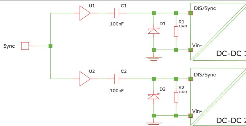
1. A suggested synchronisation circuit is shown. C1 and C2 are 100nF capacitors. D1 and D2 are schottky diodes. The capacitive isolation and close connected diode ensures that a transition from high to low is seen at the input pin even in a noisy environment or when there is a slight ground shift between devices.
