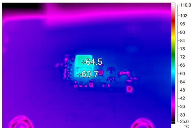
Figure 5. Thermal Image at 12V<sub>IN</sub>, 1V, 8A Output without Airflow and Heat Sink
