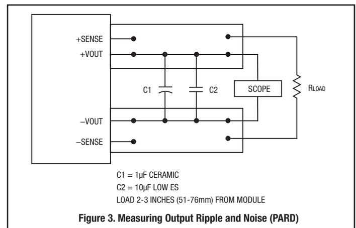
random deviations or PARD) may be reduced by adding filter elements such as multiple external capacitors. Be sure to calculate component temperature rise from reflected AC current dissipated inside capacitor ESR. Our Application Engineers can recommend potential solutions.
