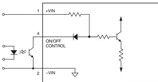
Figure 3. Driving the Negative Logic On/Off Control Pin
