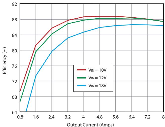
UWR-5/7-D12 Efficiency vs. Load @ 25°C Ambient
