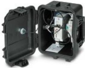
Provides a secure, cellular VPN connection to a machine network. Utilizes the Verizon cellular network.
