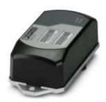
WLAN access point, client for USA and Canada, with two internal antennas for single-hole mounting, IP54, WLAN 802.11 a, b, g, n, frequency: 2.4 GHz, 5 GHz, connections: COMBICON 9 ... 32 V DC, RJ45: for LAN, web, http/ https, Command Line Interface
