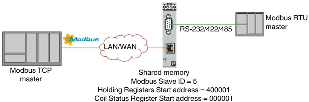
Figure 7 Modbus Master-to-Master communication using shared memory
