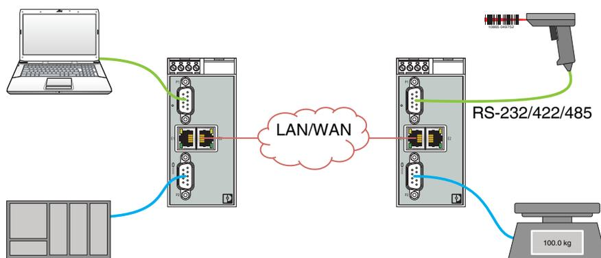
Figure 4 Serial tunneling
