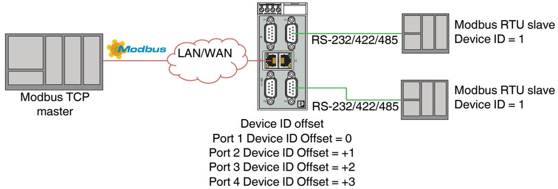
Figure 8 Serial Modbus slaves with the same Device ID on a multiport GW MODBUS TCP/RTU...
