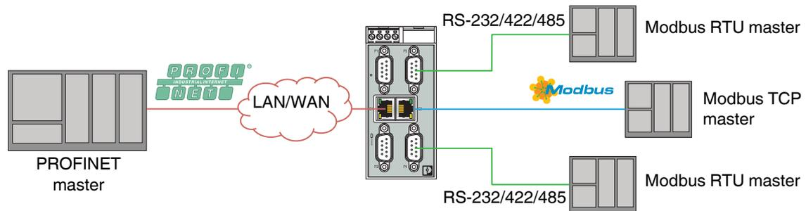
Figure 10 PROFINET to Modbus ASCII/RTU/TCP
