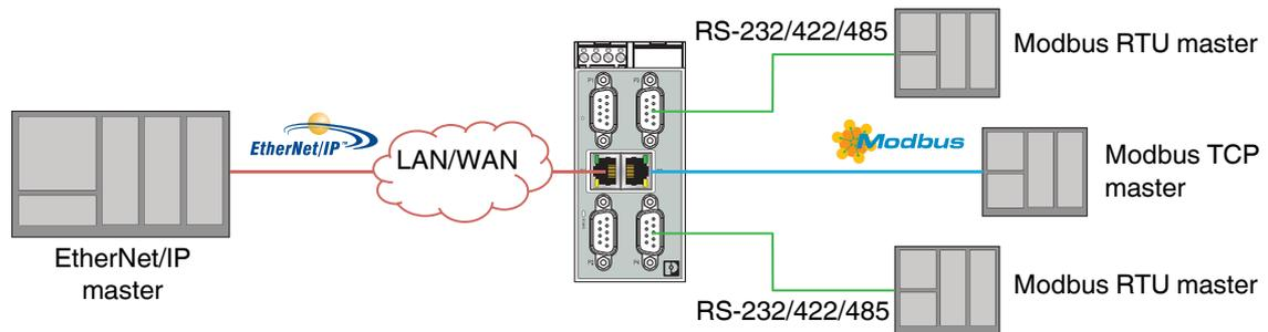
Figure 9 EtherNet/IP to Modbus ASCII/RTU/TCP
