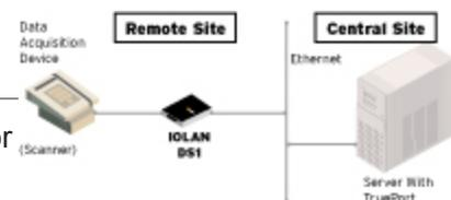
Easy to set up and manage, the IOLAN has a software selectable RS-232/422/485 interface capability which simplifies setup and eliminates mechanical tampering associated with DIP switch based products.
