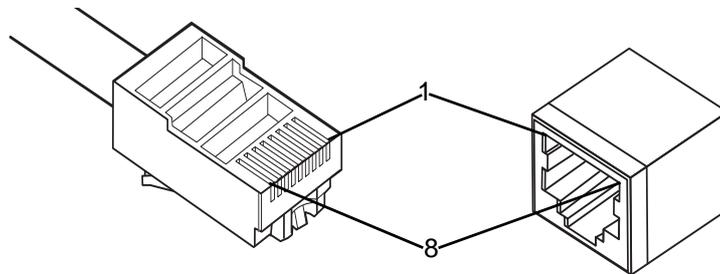
Figure 22: Ethernet Plug & Connector Pin Position
