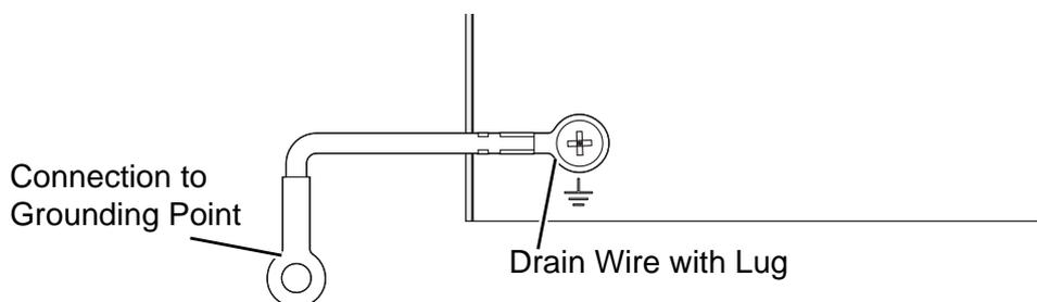
**Figure 24: Grounding Connection**
