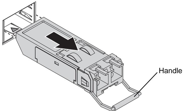
**Figure 21: Removing an SFP Transceiver**
