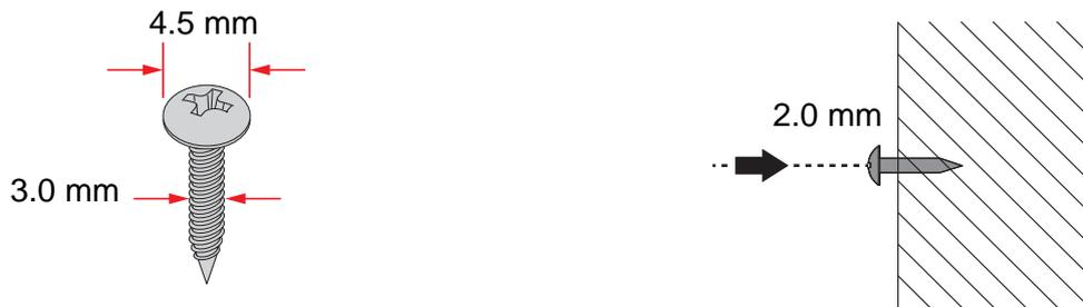
**Figure 15: Securing Wall Mounting Screws**
