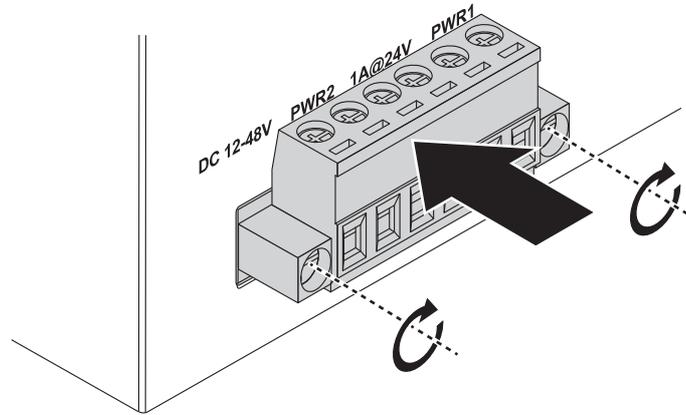
**Figure 30: Securing a Terminal Block to a Receptor**
