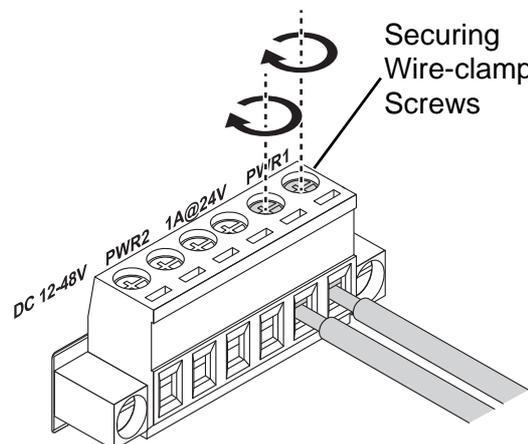
**Figure 29: Installing DC Wires in a Terminal Block**
