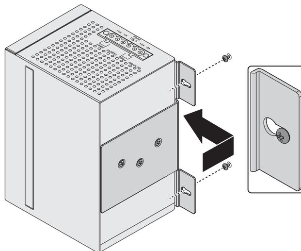
**Figure 16: Wall Mount Installation**
