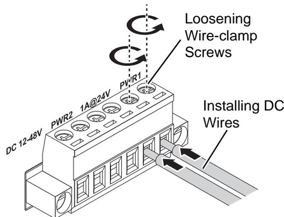
**Figure 28: Installing DC Wires in a Terminal Block**
